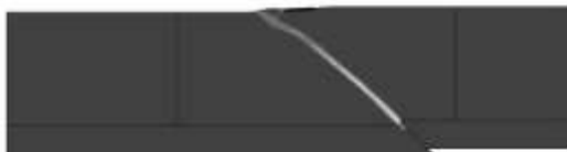
Fig. 17. Fault foundation interaction with S/B=2 (FE deformed mesh with shear strain contours)
