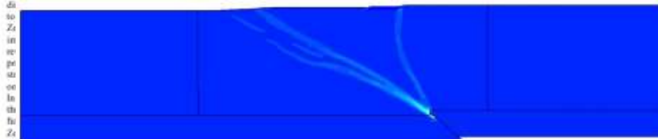
Fig. 17. Fault foundation interaction with S/B=2 (FE deformed mesh with shear strain contours)
